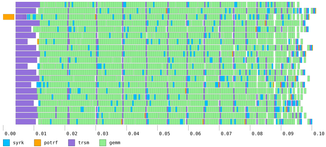
Figure 11.2: Trace of plasma_dpotrf() on Haswell:
