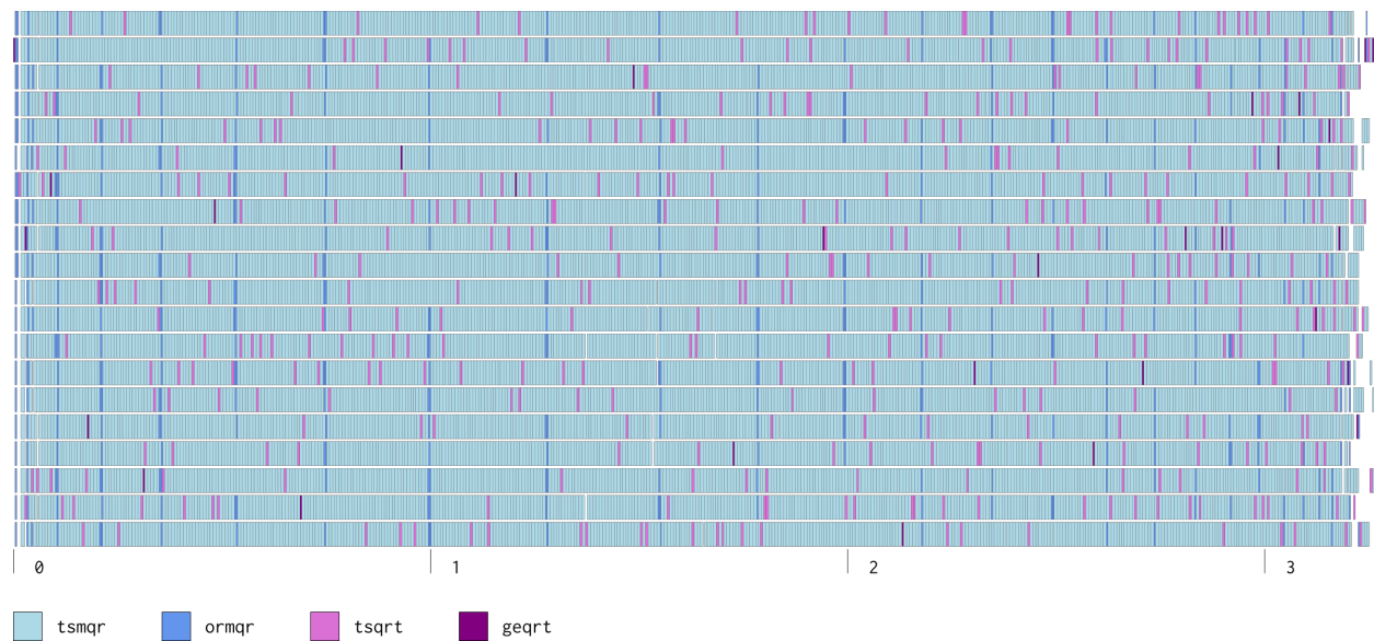
Figure 7.12: Trace of plasma_dgeqrf() on POWER8: ./test dgeqrf --dim=10000 --nb=336
