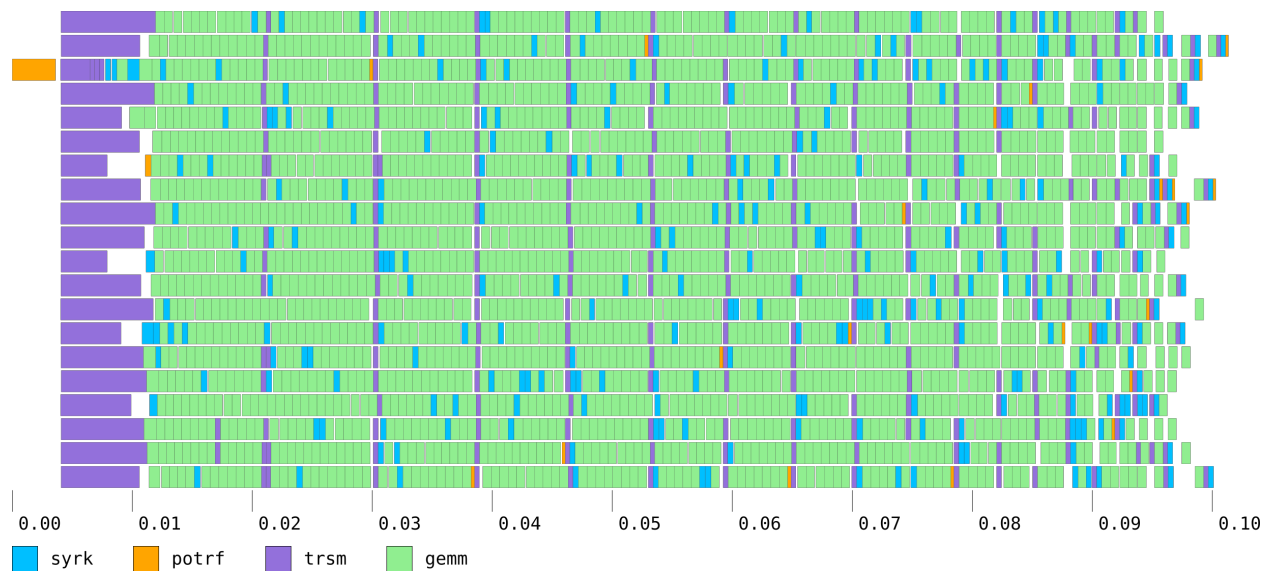
Figure 7.2: Trace of plasma.dpotrf() on Haswell: numactl --interleave=all ./test dpotrf --dim=5376 --nb=224
